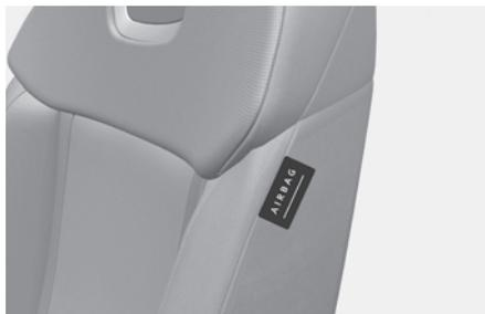
Airbag lateral central delantero (asiento del conductor)
